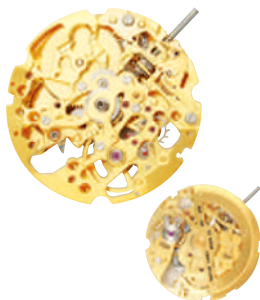
8N24 GILT height 5.55mm / 21 jewels automatic and hand winding
